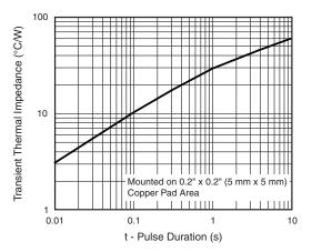
Fig. 6 - Typical Transient Thermal Impedance
