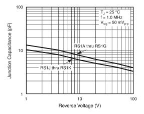
Fig. 5 - Typical Junction Capacitance
