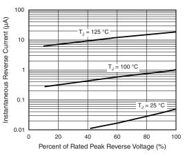
Fig. 4 - Typical Reverse Characteristics
