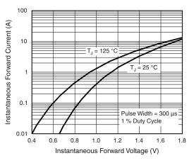
Fig. 3 - Typical Instantaneous Forward Characteristics
