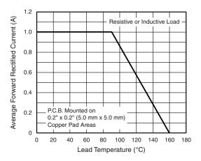
Fig. 1 - Forward Current Derating Curve
