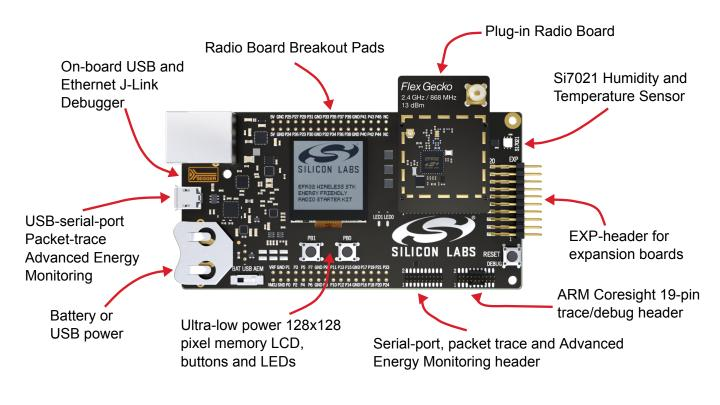
Figure 2.1. SLWSTK6061A Hardware Layout
