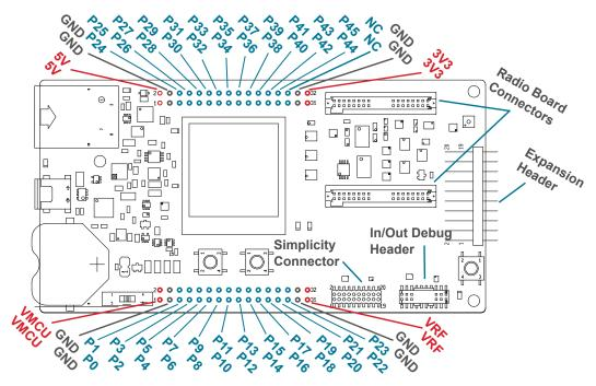
Figure 4.1. Mainboard Connector Layout
