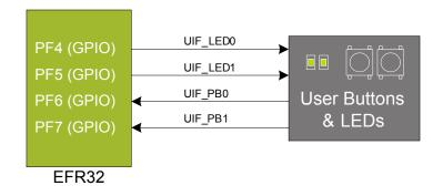
Figure 6.1. Buttons and LEDs
