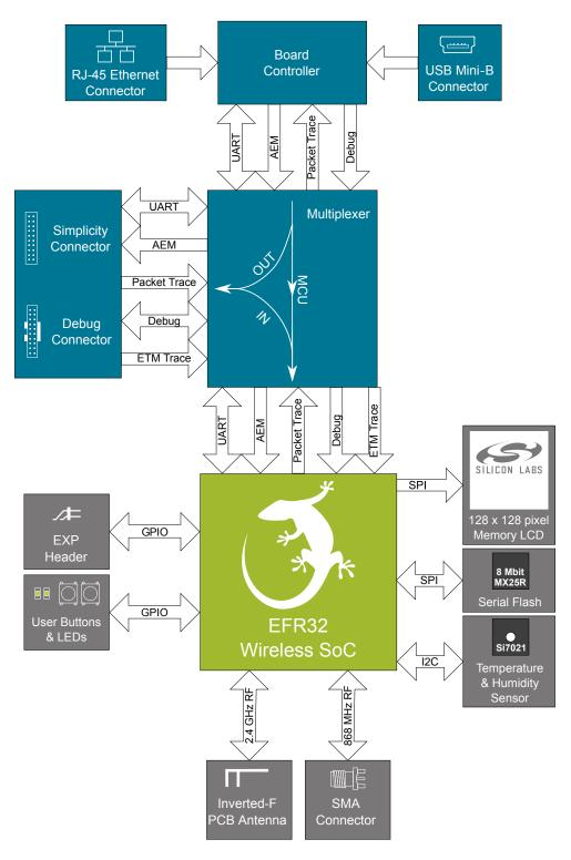
Figure 3.1. Kit Block Diagram
