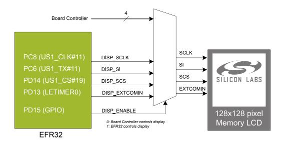
Figure 6.2. 128x128 Pixel Memory LCD
