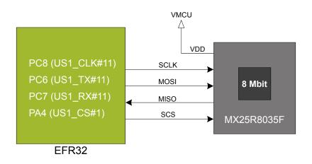
Figure 6.3. Radio Board Serial Flash
