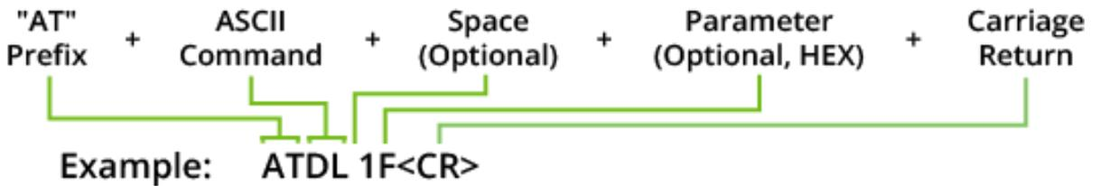
The preceding example changes the device's destination address (Low) to 0x1F.
