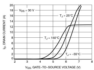
Figure 2. Transfer Characteristics
