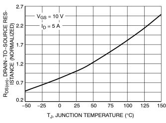
Figure 5. On–Resistance Variation with Temperature
