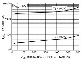
Figure 6. Drain-to-Source Leakage Current vs. Voltage
