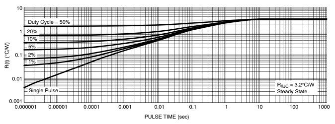
Figure 12. Thermal Impedance for NDF10N60Z
