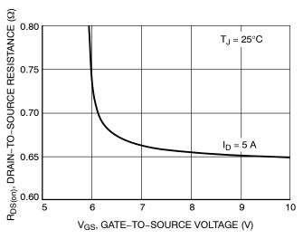
Figure 3. On-Resistance vs. Gate Voltage
