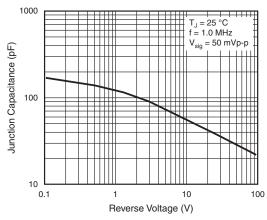
Fig. 5 - Typical Junction Capacitance
