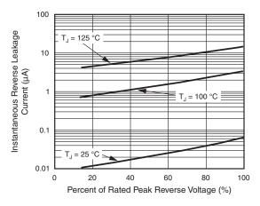
Fig. 4 - Typical Reverse Leakage Characteristics
