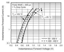
Fig. 3 - Typical Instantaneous Forward Characteristics
