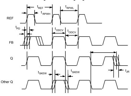
Figure 4. Zero Skew and Zero Delay Clock Driver
