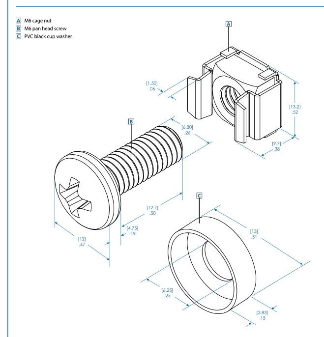
Square hole hardware kit contains 50 each M6 cage nuts, M6 pan head screws and PVC cup washers
