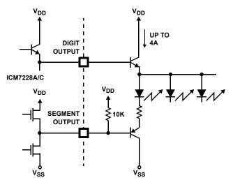
FIGURE 14. DRIVING HIGH CURRENT DISPLAY, COMMON ANODE ICM7228A/C TO COMMON ANODE
