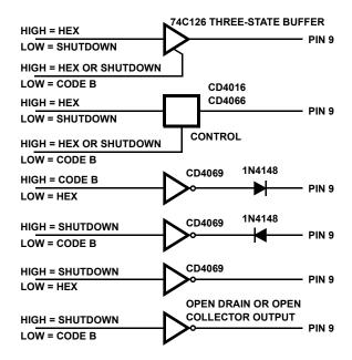
FIGURE 17. ICM7228C PIN 9 DRIVE CIRCUITS
