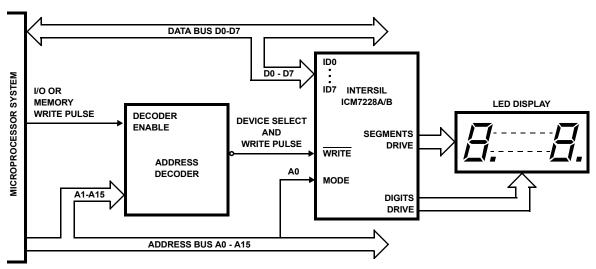
FIGURE 9. ICM7228A/B MICROPROCESSOR SYSTEM INTERFACING
