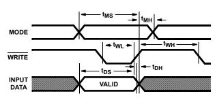
FIGURE 1. ICM7228A/B WRITE CYCLE
