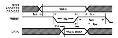
FIGURE 3. ICM7228C WRITE CYCLE
