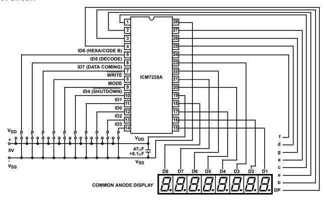
FIGURE 18. FUNCTIONAL TEST CIRCUIT #1
