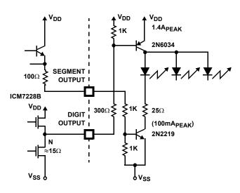
FIGURE 16. DRIVING HIGH CURRENT DISPLAY, COMMON CATHODE ICM7228B TO COMMON ANODE DISPLAY
