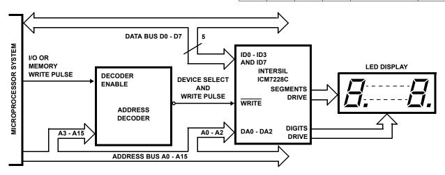
FIGURE 10. ICM7228C MICROPROCESSOR SYSTEM INTERFACING
