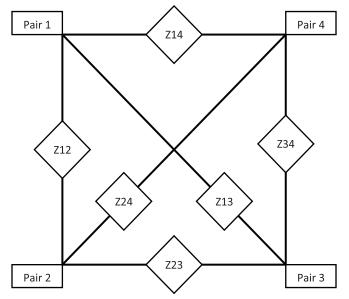
Providing those pair-to-pair transmission lines with termination matching their characteristic impedance in order to absorb the reflected wave and prevent standing wave from occurring significantly lowers parasitic interference radiation.
