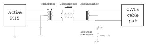
The purpose of the transformer with ratio of 1:1 is to create galvanic isolation between the cable and the system. The PHY side center tap of the transformer should connect through a capacitor to ground.
