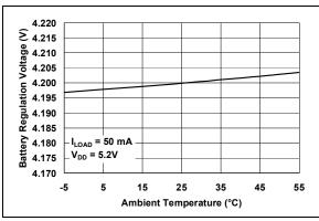
**FIGURE 2-3:** Battery Regulation Voltage  $(V_{BAT})$  vs. Ambient Temperature  $(T_A)$ .
