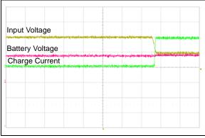
FIGURE 2-14: Overvoltage Protection Stop (50 ms/Div).
