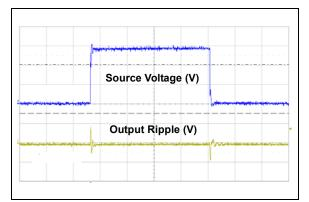
**FIGURE 2-18:** Line Transient Response  $(I_{LOAD} = 100 \text{ mA}, \text{ Output: } 1.0\text{V/Div}, \text{ Source: } 2.0\text{V/Div}).$
