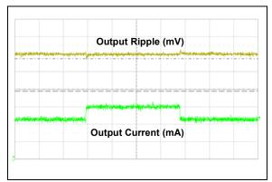
**FIGURE 2-15:** Load Transient Response  $(I_{LOAD} = 50 \text{ mA}, \text{ Output: } 100 \text{ mV/Div}, Time: 100 <math>\mu$ s/Div).
