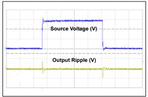
**FIGURE 2-17:** Line Transient Response  $(I_{LOAD} = 10 \text{ mA}, \text{ Output: } 1.0 \text{V/Div}, \text{ Source: } 2.0 \text{V/Div}).$
