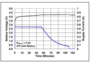
FIGURE 2-16: Complete Charge Cycle (875 mAh Li-Ion Battery.
