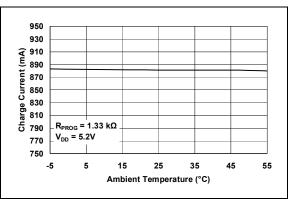
**FIGURE 2-11:** Charge Current ( $I_{OUT}$ ) vs. Ambient Temperature ( $T_A$ ).
