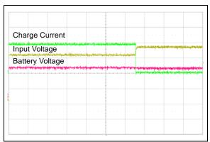
FIGURE 2-13: Overvoltage Protection Start (50 ms/Div).
