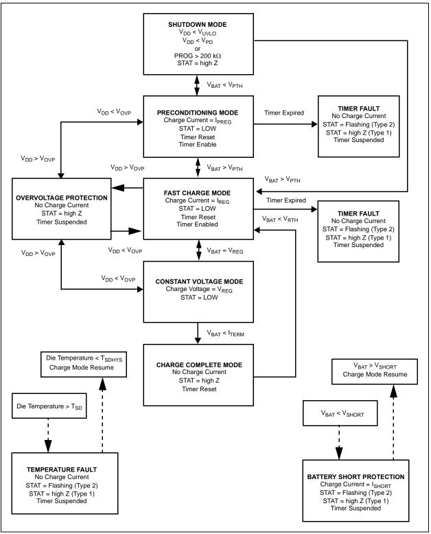
FIGURE 4-1: The MCP73113/4 Flowchart.
