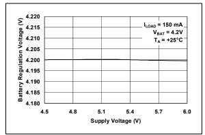
**FIGURE 2-2:** Battery Regulation Voltage (V<sub>BAT</sub>) vs. Supply Voltage (V<sub>DD</sub>).
