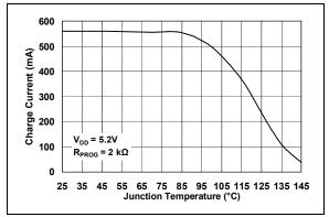
**FIGURE 5-1:** Charge Current  $(I_{OUT})$  vs. Junction Temperature  $(T_J)$ .
