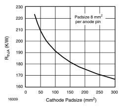
Fig. 5 - Thermal Resistance Junction Ambient vs. Cathode Padsize
