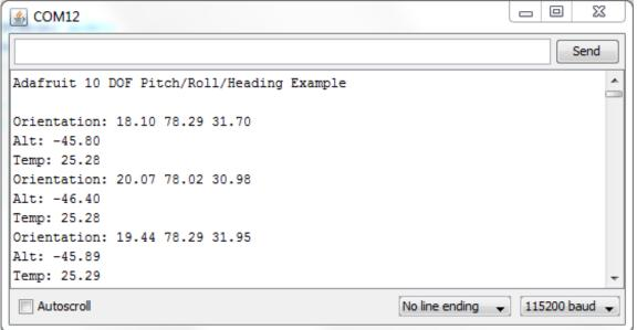
In this case, we can see that the roll is about 18°, the pitch is about 78° and the heading or yaw is about 32°, and the sketch will keep updating itself with the latest values at whatever
