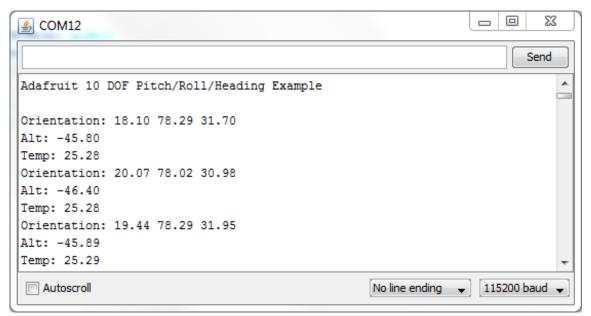
This raw data shows the main orientation data, consisting of 'roll', 'pitch' and 'heading' (or 'yaw) in degrees, followed by the current altitude and temperature if you are are using the 10-DOF breakout (the 9-DOF and LSM9DSO breakouts can't measure altitude).
