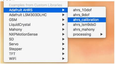
Be default this is setup for the sensors found on the Adafruit 9DOF and 10DOF breakouts, but can be adjusted to work with any accelerometer, magnetometer and gyroscope that is based on the Adafruit Unified Sensor system (http://adafru.it/dGB).
