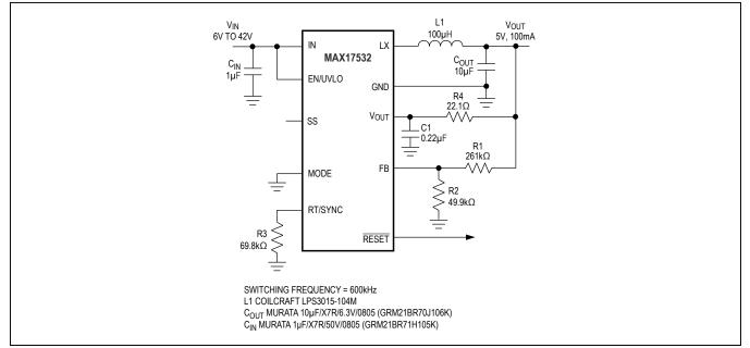
Figure 8. Small Footprint 5V, 100mA Regulator
