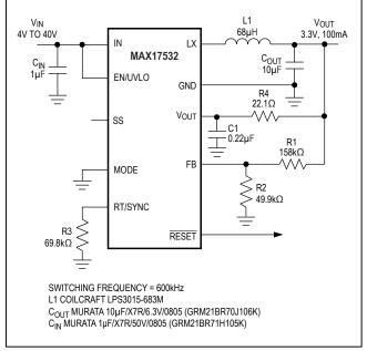
Figure 9. Small Footprint 3.3V, 100mA Regulator
