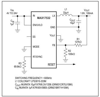
Figure 10. Small Footprint 1.8V, 100mA Regulator
