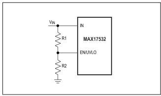
Figure 2. Adjustable EN/UVLO Network
