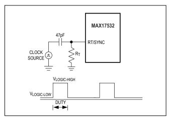
Figure 1. Synchronization to an External Clock
