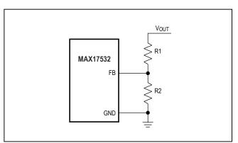
Figure 3. Setting the Output Voltage
