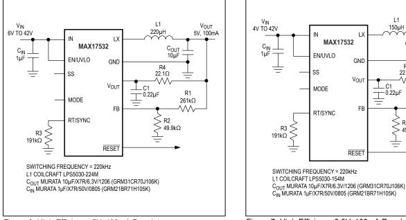
Figure 6. High-Efficiency 5V, 100mA Regulator
