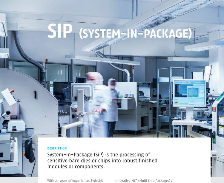
with 25 years of experience, Swissbit successfully uses advanced packaging technologies to achieve the smallest form factors and to build multi-chip-packages. With this electronic integration approach, our products provide more functionality inside one package, various functional blocks (RF, digital, sensors, security, and memory) as well as passive components are combined. Having all necessary capabilities inhouse we have the best design for reliability, test and production.
