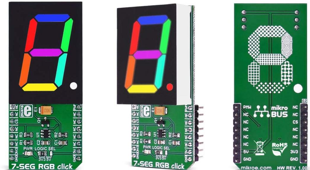
**7-SEG RGB click** carries a full-color single 7 segment digit display. The click is designed to run on either 3.3V or 5V power supply. It communicates with the target microcontroller over the CS, and PWM pin on the mikroBUS™ line.
