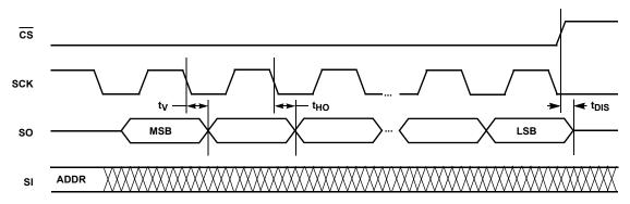
FIGURE 8. OUTPUT TIMING
