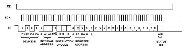
FIGURE 6. FOUR-BYTE INSTRUCTION SEQUENCE (READ STATUS REGISTERS)
