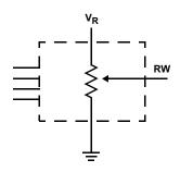
FIGURE 12. THREE-TERMINAL POTENTIOMETER; VARIABLE VOLTAGE DIVIDER
