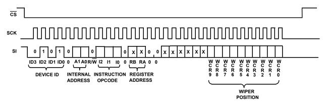
FIGURE 5. FOUR-BYTE INSTRUCTION SEQUENCE (WRITE OR READ FOR WCR OR DATA REGISTERS)
