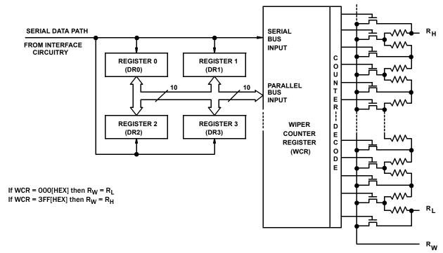
FIGURE 3. DETAILED POTENTIOMETER BLOCK DIAGRAM
