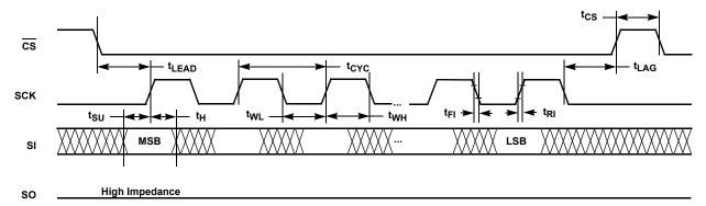
FIGURE 7. INPUT TIMING
