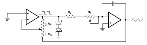
$\begin{aligned} & \text{FREQUENCY} \propto R_1, \, R_2, \, C \\ & \text{AMPLITUDE} \propto R_A, \, R_B \end{aligned}$
