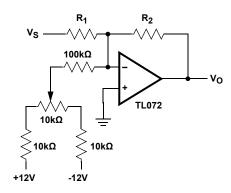
FIGURE 16. OFFSET VOLTAGE ADJUSTMENT
