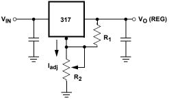
$V_0 (REG) = 1.25V (1+R_2/R_1)+I_{adj} R_2$
