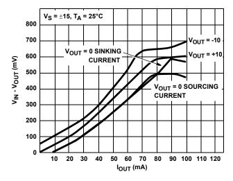
FIGURE 17. VIN - VOUT VS IOUT
