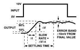
FIGURE 3. SETTLING TIME AND SLEW RATE
