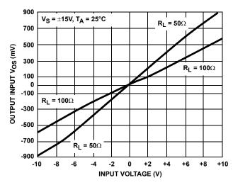
FIGURE 15. GAIN ERROR vs INPUT VOLTAGE
