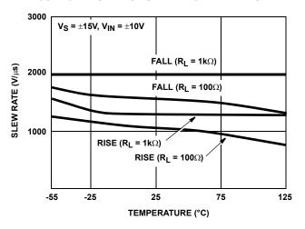
FIGURE 11. SLEW RATE vs TEMPERATURE
