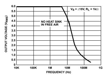
FIGURE 24. OUTPUT SWING vs FREQUENCY (NOTE)
