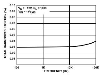
FIGURE 21. TOTAL HARMONIC DISTORTION vs FREQUENCY
