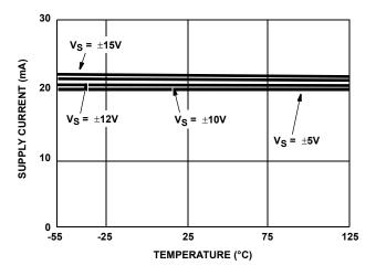
FIGURE 10. SUPPLY CURRENT vs TEMPERATURE
