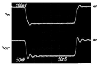
$T_A = 25$ °C,  $R_S = 50\Omega$ ,  $R_M = R_L = 50\Omega$
