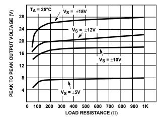
FIGURE 23. OUTPUT VOLTAGE SWING vs LOAD RESISTANCE
