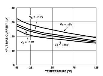
FIGURE 9. INPUT BIAS CURRENT vs TEMPERATURE
