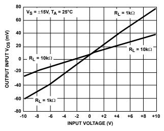
FIGURE 14. GAIN ERROR vs INPUT VOLTAGE
