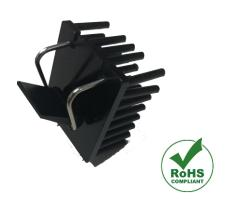
Wakefield-Vette introduces the Omni series forged pin-fin heat sink (Pat. Pending). This series heat sinks offer all-in-one solution, compact design with universal cam clip system for TO-220, TO-247, TO-264 and others package compatible devices. This powerful heat sink can be thru-hole soldered onto PCBs. The pin fins make the minimum flow impedance. It is the ideal type of heat sink for high power and small size (1U or 2U) electronic packaging with natural and forced convection cooling
