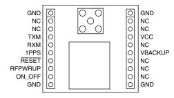
Figure 4: EVM-GPS-R4 Pin Assignments
