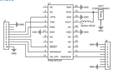
Figure 6: EVM-GPS-R4 Schematic
