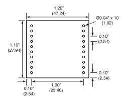
Figure 5: EVM-GPS-R4 PCB Layout Dimensions
