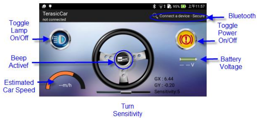
Figure 7 GUI of Smart Car application on Android device
