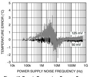
Figure 13. Remote Temperature Error vs. Power Supply Noise
