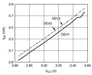
Figure 6. Supply Current vs. Voltage
