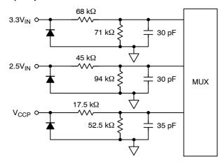
Figure 14. Internal Structure of Analog Inputs
