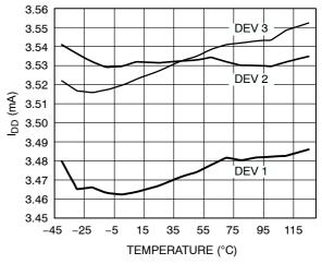
Figure 3. Supply Current vs. Temperature
