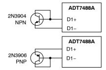
Figure 16. Connections for NPN and PNP Transistors
