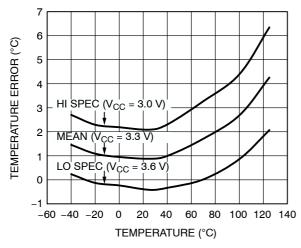
Figure 4. Local Temperature Error
