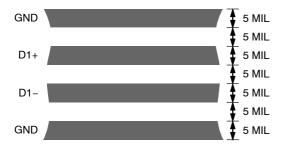
Figure 17. Arrangement of Signal Tracks
