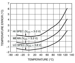
Figure 7. Remote Temperature Error
