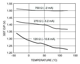
Figure 5. SST O/P Level vs. Temperature
