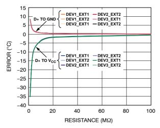
Figure 8. Remote Temperature Error vs. PCB Resistance
