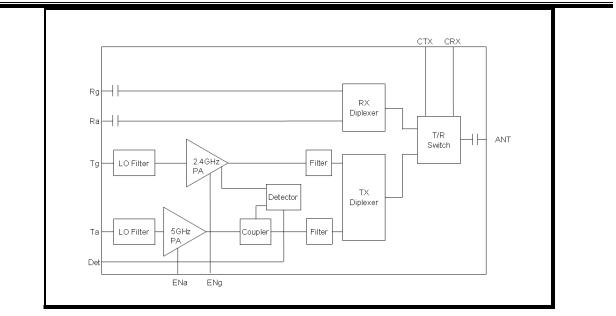
Figure 1: SE2548A Functional Block Diagram
