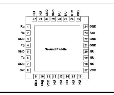
Figure 2: SE2548A Pin Out (Top View Through Package)
