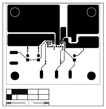
Figure 2. MAX17532 5V EV Kit (µMAX) PCB Layout— Component Side
