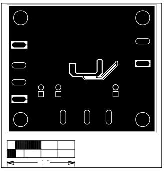
Figure 3. MAX17532 5V EV Kit ( $\mu$ MAX) PCB Layout—Solder Side
