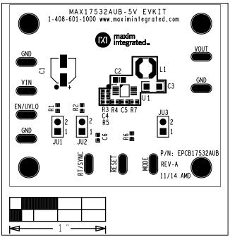
Figure 1. MAX17532 5V EV Kit (µMAX) Component Placement Guide—Component Side
