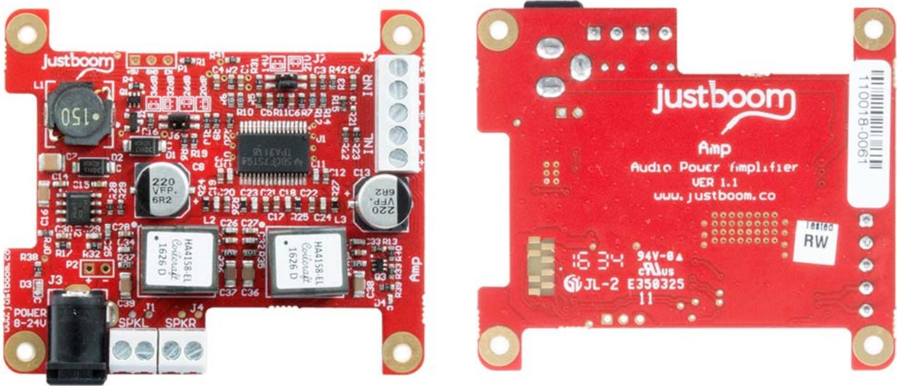
The JustBoom Amp is a standalone high quality audio power amplifier that is designed to either stack on top of the JustBoom DAC / DAC HAT or alternatively take a line level input. We've designed the JustBoom Amp to be simple to use – with no soldering required and all the mounting hardware already provided, this is a true plug and play device
