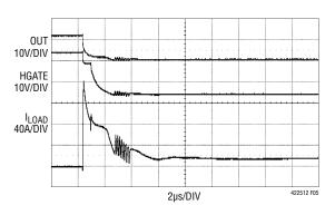
Figure 5. Severe Short-Circuit on 12V Output
