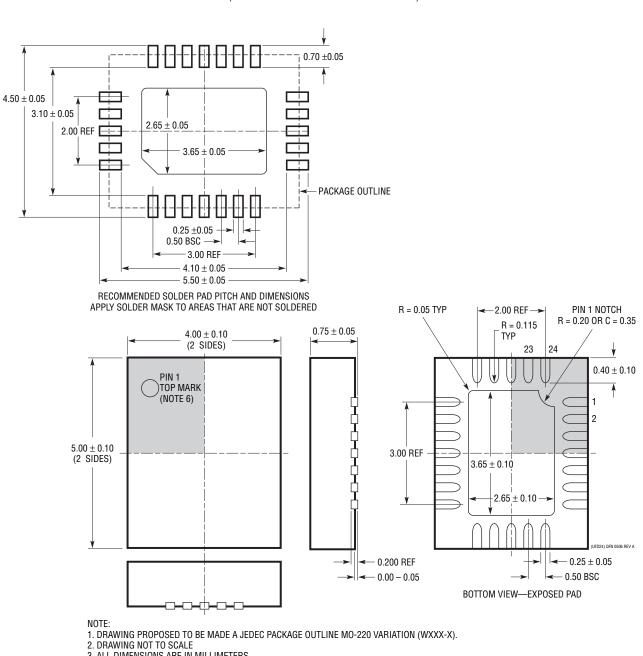
**UFD** Package 24-Lead Plastic QFN ( $4mm \times 5mm$ ) (Reference LTC DWG # 05-08-1696 Rev A)
