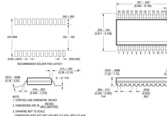
**GN Package** 24-Lead Plastic SSOP (Narrow .150 Inch) (Reference LTC DWG # 05-08-1641)
