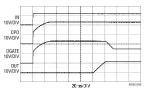
Figure 2. Ideal Diode Controller Start-Up Waveforms
