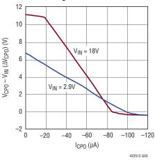
**Diode Gate Voltage vs Current** 12  $V_{OUT} = V_{IN} - 0.1V$ 10 Vdgate – Vin (ΔVdgate) (V) 8 V<sub>IN</sub> = 18V 6 4  $V_{IN} = 2.9V$ 2 0 -2 -20 -80 0 -40 -60 -100 -120 IDGATE (µA)
