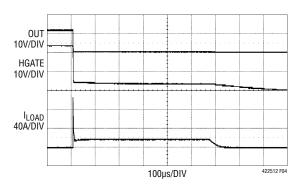
Figure 4. Overcurrent Fault on 12V Output
