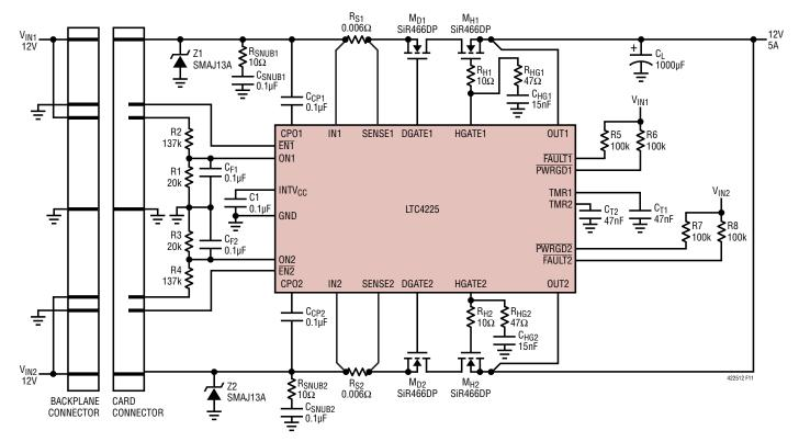
Figure 11. Card Resident Application with the Output Diode-ORed
