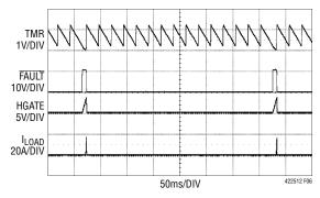
Figure 6. Auto-Retry Sequence After a Fault
