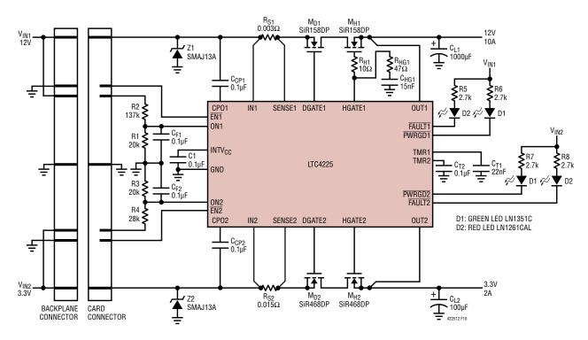
Figure 10. Plug-In Card Supply Holdup Using Ideal Diode at 12V and 3.3V Input Supplies
