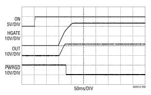
Figure 3. Hot Swap Controller Power-Up Sequence
