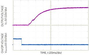
Figure 4. Typical Start-Up Using negative Remote On/Off;  $C_{o,\text{ext}}$  = 440 $\mu F.$
