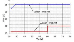
**Figure 12. Output Voltage Trim Limits vs. Input Voltage.** See Figure 12 for the allowed input to output range when using trim. If not using the trim down feature, leave the TRIM pin open.
