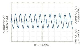
Figure 2. Typical Output Ripple and Noise at Room Temperature and 48Vin;  $I_{o}$  =  $I_{o,max};$   $C_{o,ext}$  =  $440\mu F.$
