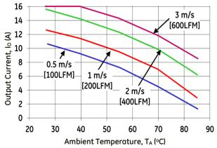
Figure 20. Derating Output Current vs. local Ambient temperature and Airflow, No Heatsink, Vin=48V, airflow from Vi(-) to Vi(+).
