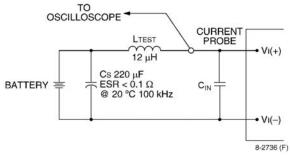
Note: Measure the input reflected-ripple current with a simulated source inductance (LTEST) of 12  $\mu$ H. Capacitor CS offsets possible battery impedance. Measure the current, as shown above. Figure 7. Input Reflected Ripple Current Test Setup.
