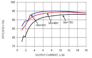
Figure 1. Converter Efficiency versus Output Current.
