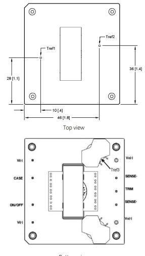
Bottom view Figure 18. Case (TREF) Temperature Measurement Location
