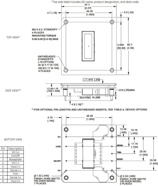
JNCW016A0R Orca Series; DC-DC Converter Power Modules 36–75 Vdc Input; 28.0Vdc Output; 16Adc Output
