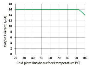
Figure 19. Output Power Derating for JNCW016A0R in Conduction cooling (cold plate) applications;  $T_{\alpha}$  <70°C adjacent to module;  $V_{IN} = V_{IN,NOM}$
