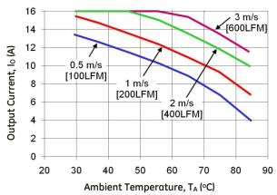
Figure 21. Derating Output Current vs. local Ambient temperature and Airflow, 0.5" Heatsink, Vin=48V, airflow from Vi(-) to Vi(+).
