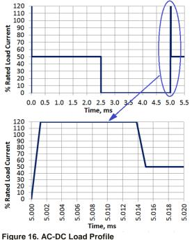
The output voltage peak deviation shall not exceed the peak values listed in the Electrical Specifications Table.
