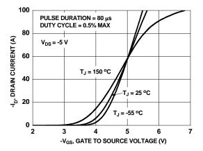
Figure 5. Transfer Characteristics
