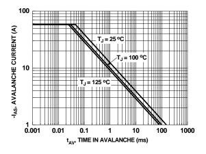
Figure 9. Unclamped Inductive Switching Capability
