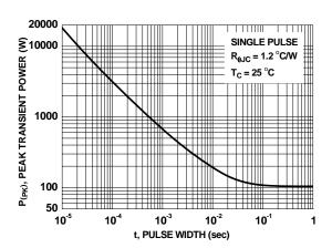
Figure 12. Single Pulse Maximum Power Dissipation
