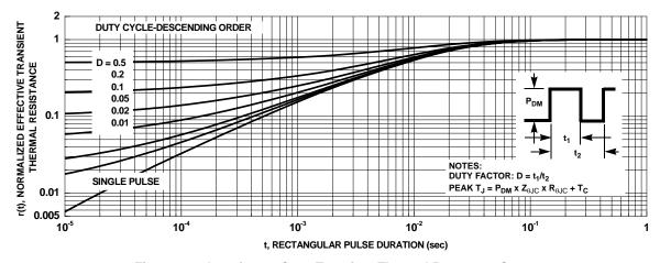
Figure 13. Junction-to-Case Transient Thermal Response Curve
