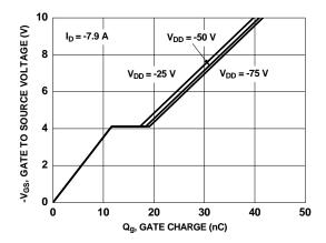
Figure 7. Gate Charge Characteristics
