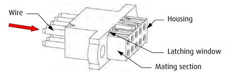
Push the contact and wire forward into the housing in the direction as shown, taking the load off of the contact latching feature on the contact.
