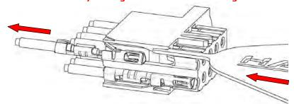
Whilst keeping the tool in place, gently pull the wire and contact in the direction shown, to remove them from the housing.
