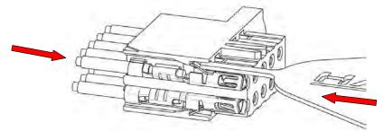
Slide the probe down the side of the mating section of the crimp housing, into the latching window of the crimp to be removed.
