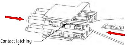
feature Push the tool to depth. Do not forcefully insert, insert on an angle, or insert with a twisting action. It may damage the tool or the housing
