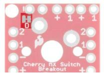
Like the resistor, the breakout shorts across the diode. Cutting this jumper removes the short and functionally adds the diode to the circuit.
