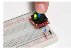
Now actuate the switch, and watch for the LED to illuminate.
