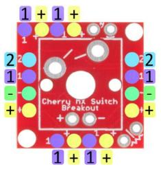
The pair of headers on the left and right sides of the board **break out all four pins**. These are intended for primary use. You can solder male pins into both of these headers, and plug the switch into a breadboard.
