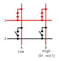
While the diode does prevent ghosting, it does place certain restrictions on your button-press detection. It forces the switch contact on the diode's anode (positive) side to be at a higher voltage than the other contact, as the switch can only conduct meaningful current in one direction.
