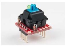
You'll also need to **cut the "D" jumper** on the back side of the board – otherwise the diode will be shorted over. (This may be easier if you do it before soldering anything.)
