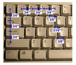
Typical keyboard row offsets. (Image courtesy of The PC Guide.)
