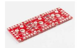
There's not an easy method to soldering boards together. You'll probably need wire strippers to split and cut solid-core wire into tiny (~3/8") pieces. A third hand can be a big-time help keeping boards stationary while you solder the little wires in place.
