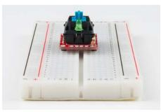
The pair of headers breaking *only* the LED anode and switch contact 1 are designed for keypad matrices, where multiple boards are connected in row/column pairs. More on this later in the tutorial.
