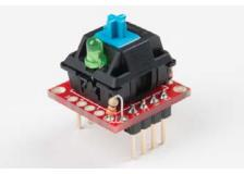
You'll also need to **cut the "R" jumper** on the back side of the board, which might be easier to do before you solder anything. A hobby knife and a steady hand should do the trick.
