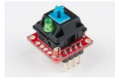
In addition to breaking out the switch contacts to breadboard-compatible headers, the breakout also provides access to an optional switch-mounted LED. Plus, the pin break-outs are designed with keyboard matrix-ing in mind, so you can interconnect as many boards as you'd like into a row-column configuration, keeping the I/O-pin requirements as low as possible.
