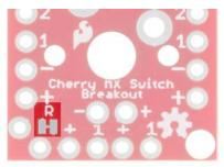
By default, the board has a short across the current-limiting resistor. Cutting this jumper removes the short, and functionally adds the resistor to the circuit.
